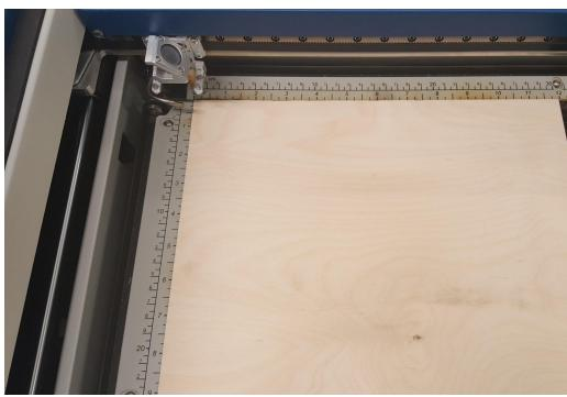
To lower bed for material clearance press "X/Y Off", then Go.
